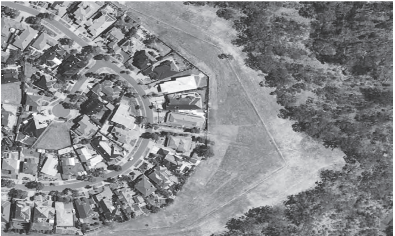
Figure 3. Providing a buffer between existing vegetation and a subdivision to reduce bushfire risk.
